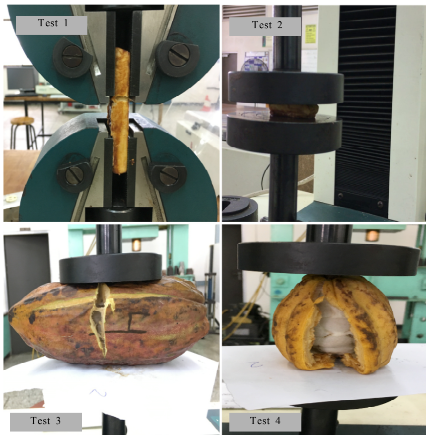
Figure 1. Universal testing machine configuration for tests 1–4
